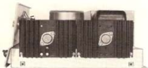
Each of the conservatively rated output transistors is individually mounted in a large heat sink to rapidly dissipate heat and improve performance.
